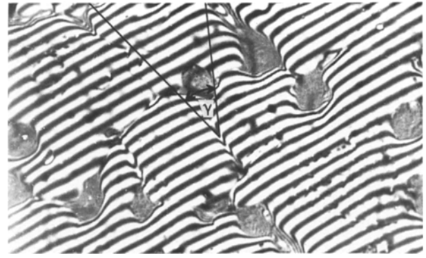
Figure 3 Interference patterns to obtain the groove angle \psi of ZrO_2 in argon ( T = 1523 K, t = 10 h, \lambda = 589 nm, m = 605 \times ).
